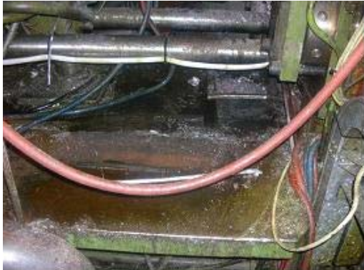
Fig 10: Conventional product. Note pool of oil below piston
