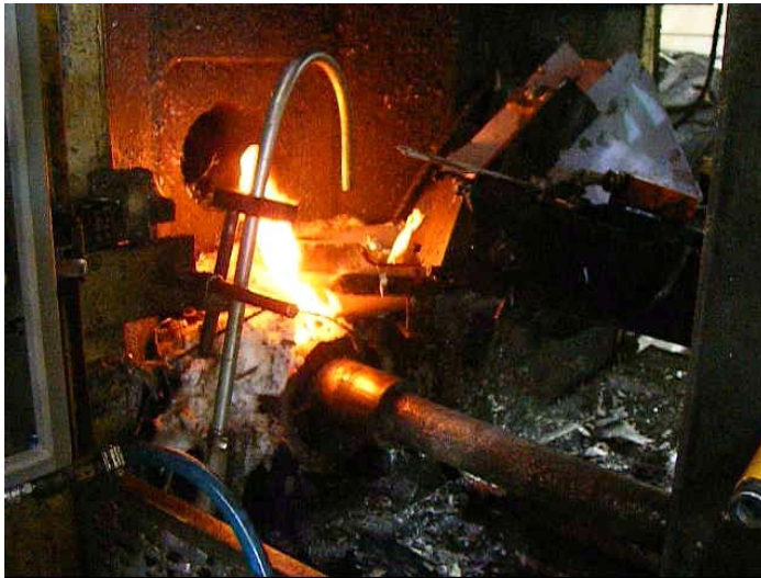
Fig 4: Flames from shot sleeve
