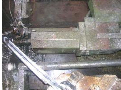
Fig 11: High efficiency lube. No spillage below piston
