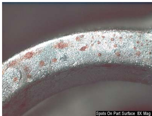
Fig 3: Stain on casting
