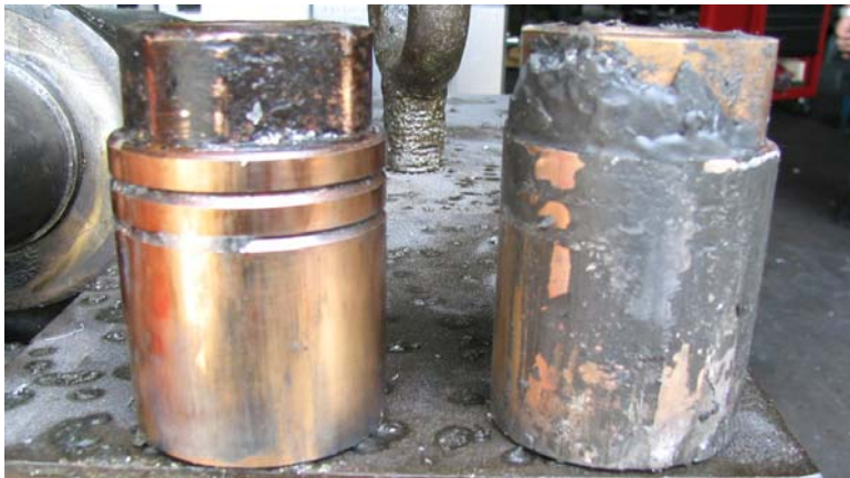
Fig 8: Comparison of Chem-Trend plunger lube tip (left) and the competitive product tip (right).
